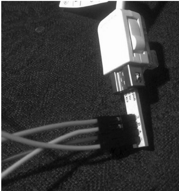
Figure 12-5. Correct positioning of Wiichuck adapter
