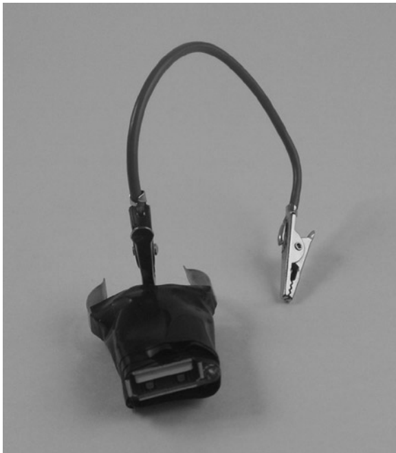
Figure 10-5. Hacked car charger
