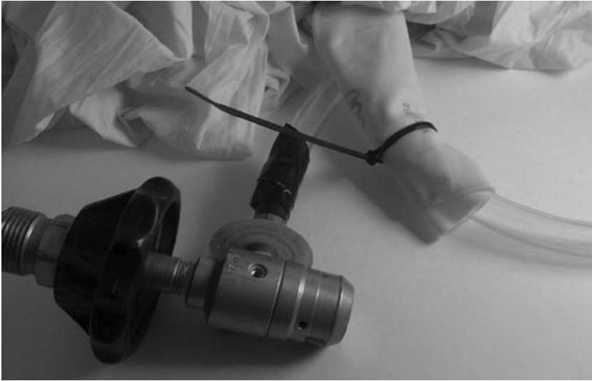
Figure 11-2. Regulator-to-balloon neck setup
