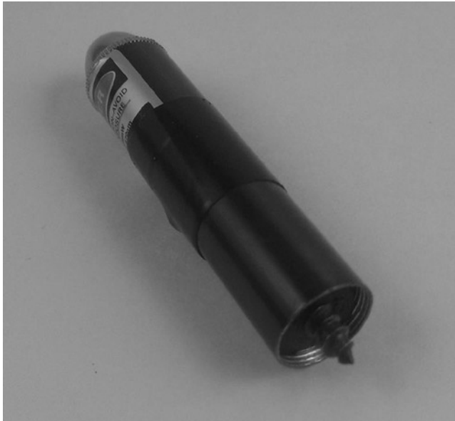
Figure 9-6. Completed laser pointer mechanism
