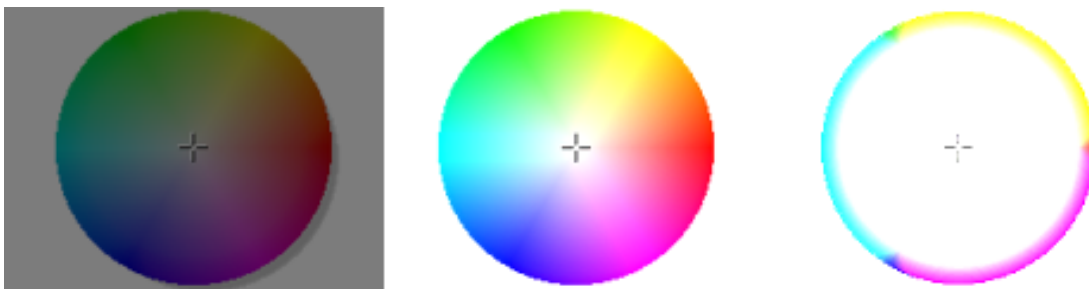
The color wheel with brightness values of 0.5, 1.5, and 10, respectively
