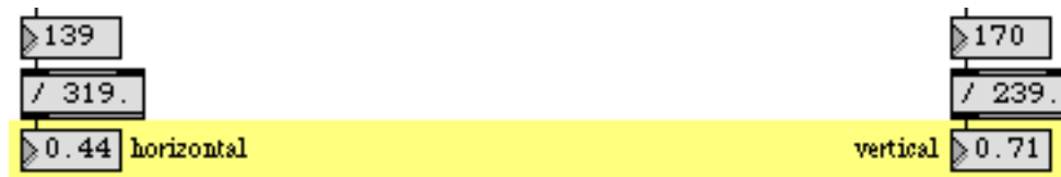
Scale the location coordinates into the range 0-1, for use elsewhere in the patch.
