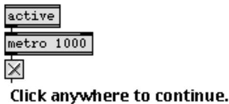
Blinking text by switching between items of a menu in Label mode
