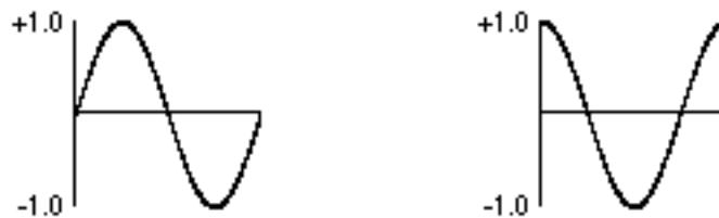
A sine wave offset by a quarter cycle is a cosine wave
