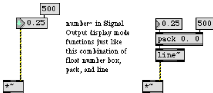
number~ can send a linear ramp signal from its old value to a new value
